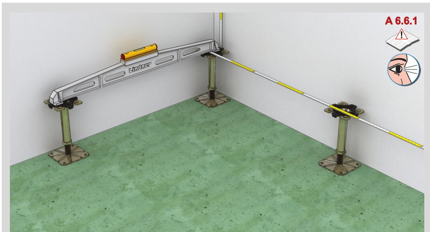
Figure 13 Installation of the further pedestals for the first raised floor panel
