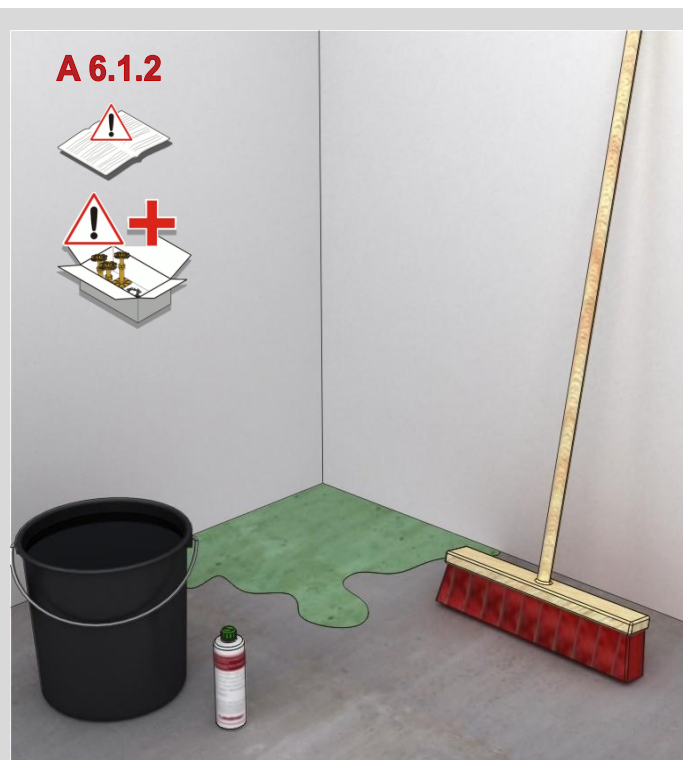
Figure 5 Application of the subfloor sealant
